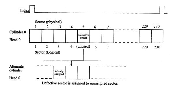
Figure 6.8 Alternate cylinder assignment
